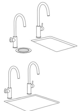
HydroTap Arc can be installed over sink or optional font
